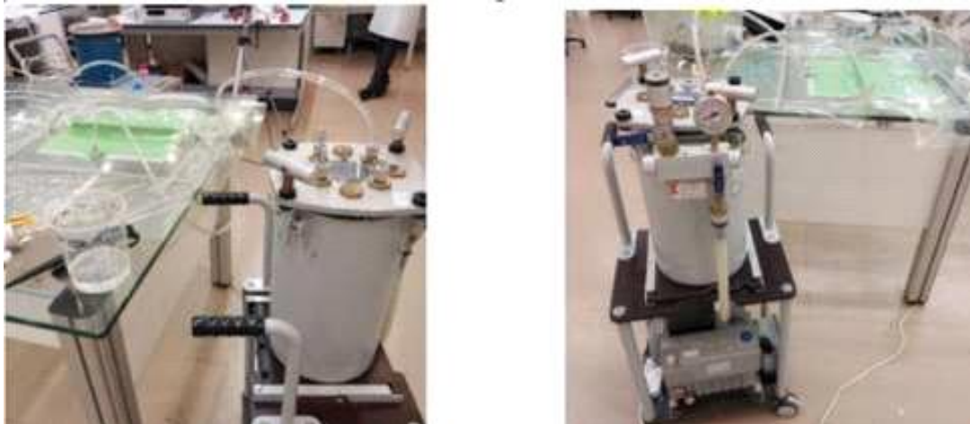
Figure 1a and 1b : Thermoset resin injection and uni-directional flow mesh layup through vacuum pressure
