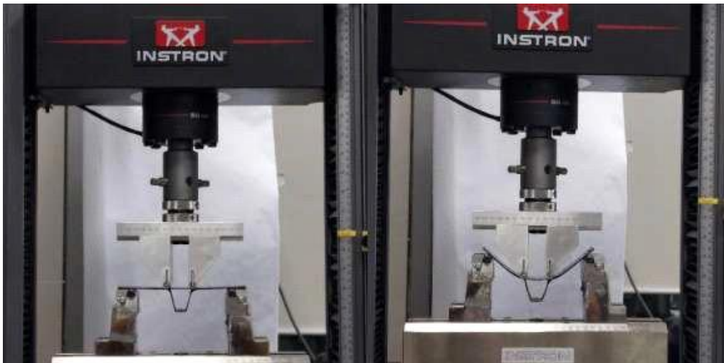
Figure 2a and 2b : Three point testing experimental setup and point of delamination when specimen fails under loading
